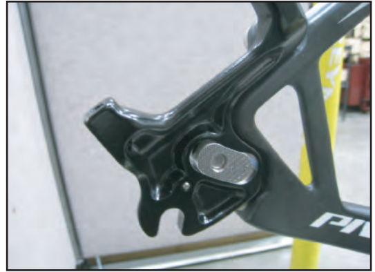
NDS dropout installed like image. Flip nut 180 degrees to extend travel.
