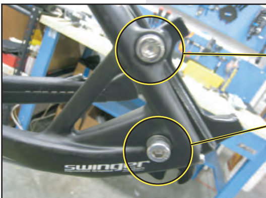
Torque bolts as shown. Use Blue Loctite.
