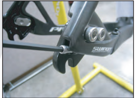
Use 4mm hex key to adjust chain tension. Count indexed "clicks" on each side to match DS/NDS dropout distance.
