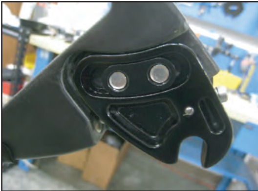
DS dropout installed.
